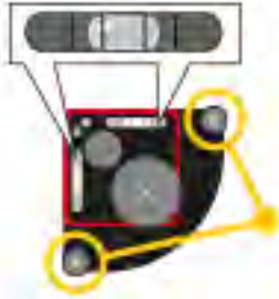
Level the laser transmitter
