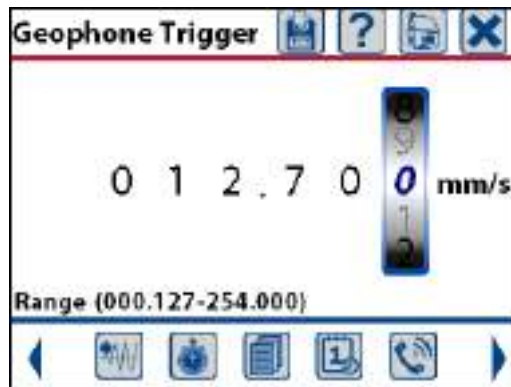
Geophone Trigger Level Set to 12.7 mm/s
