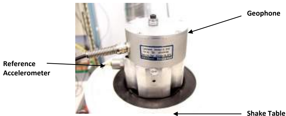
Geophone Secured to Shake Table
