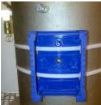
Micromate Attached with Plastic Tie-wraps
