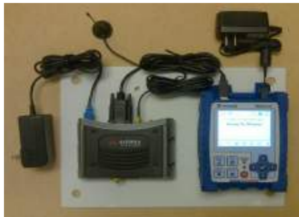
Placement of Modem, Micromate and Cables
