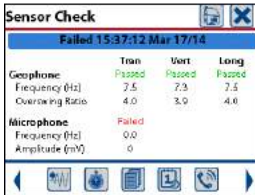
Sensor Check – Microphone Failing
