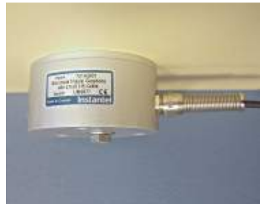
Geophone Mounted to the Ceiling
