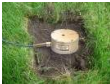
Geophone - Spikes Installed Geophone - Spiked in Ground Geophone - Partially Buried
