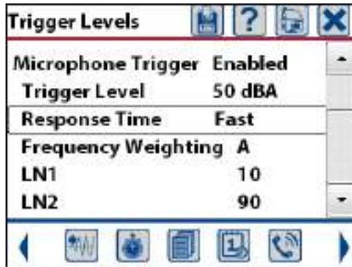
Sound Level Microphone Response Time set to Fast
