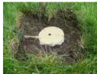
Geophone - Spikes Installed Geophone - Spiked in Ground Geophone - Partially Buried
