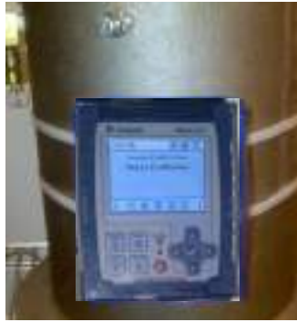
Micromate Attached with Plastic Tie-wraps
