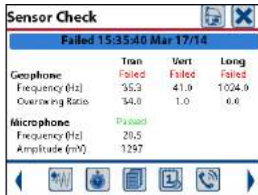
Sensor Check – All Geophones Failing
