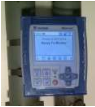
Micromate Attached with Metal Straps
