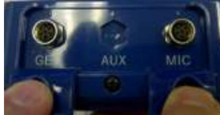
Dust Caps Pulled Back to Access Connectors
