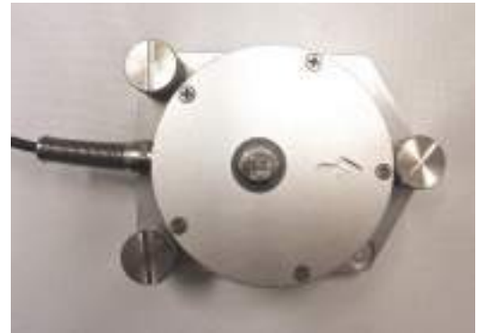
Geophone Mounted with a Leveling Plate
