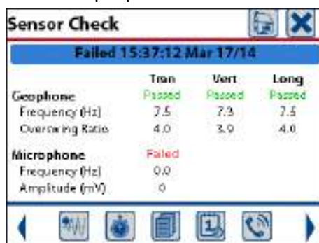
Failing Microphone Sensor Check
