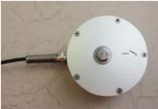
Geophone Bolted to a Floor
