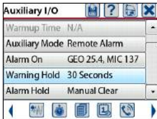
Sample Remote Alarm Setup
