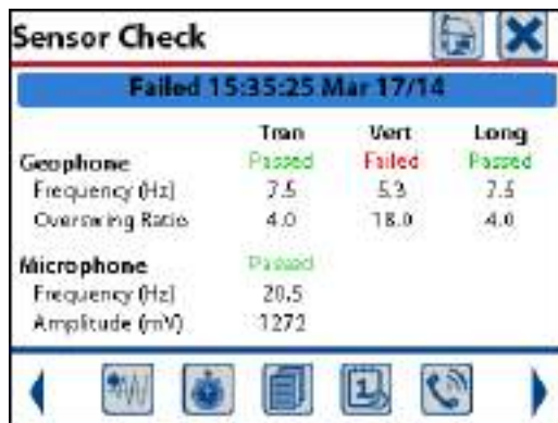
Sensor Check – Failing Vert Sensor
