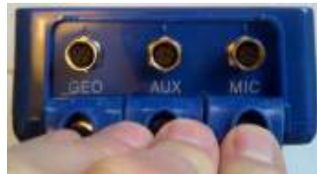
Dust Caps Pulled Back to Access Connectors
