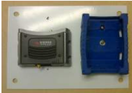
Modem and Protective Boot Secured
